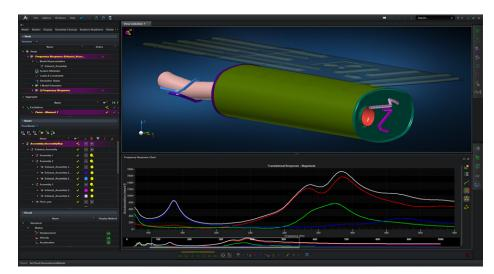
Adjust mode contributions and immediately view impact on frequency responses through an integrated Modes Configuration tool
